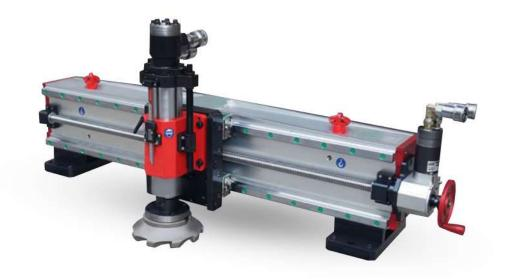
MRY Series line milling machine is 2 axis line milling machine, it can be used on heat exchangers, pump and motor pads, steel mill stands, ship building, turbine split lines and many more applications. • X Axis Stroke:1500mm (59.0") • Z Axis Stroke:250mm (10.0")
